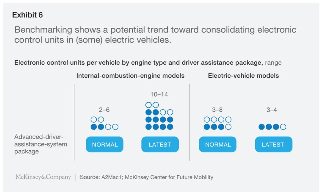
An OEM's decision for a centralized or decentralized ECU architecture can be a strategic question and will be driven by different factors. One reason for a centralized approach may be the choice to “own” a key control point in the vehicle by becoming an integrator, which could facilitate advanced software development and potentially open up new revenue streams, for example, from over-the-air updates.
